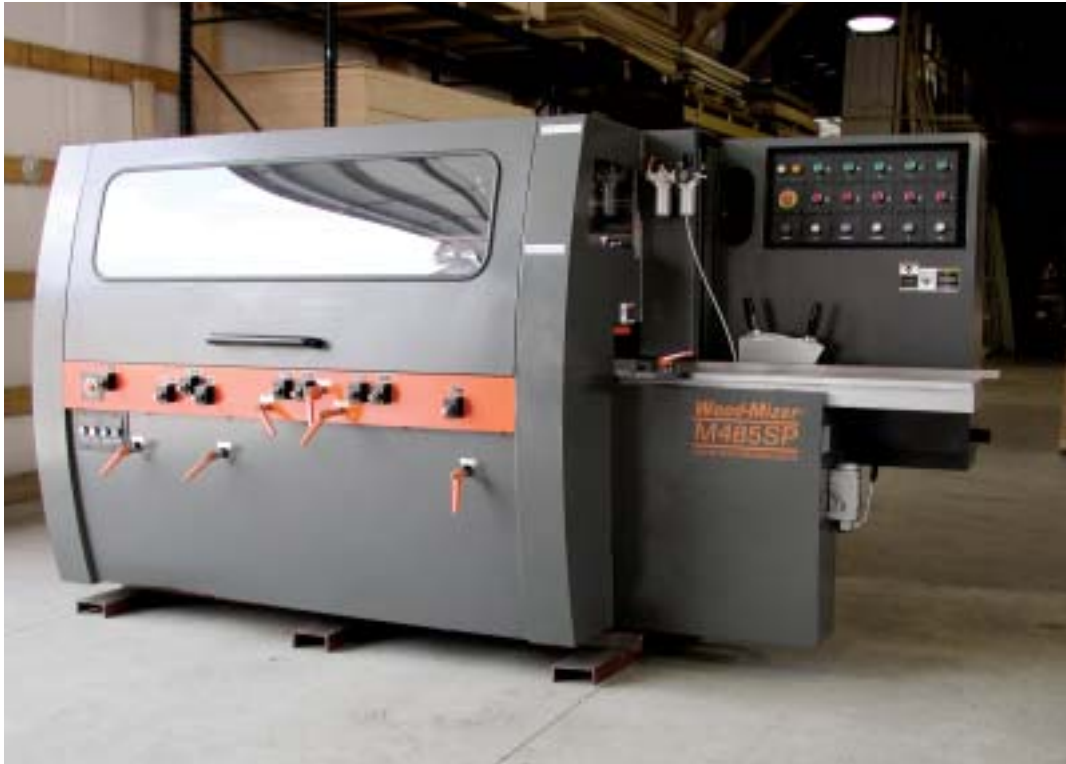
Left The Wood-Mizer Molder provides the proper tool to make trim and moldings for the home
