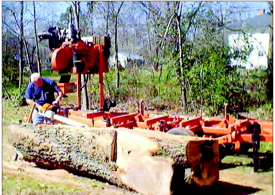
Prepping large log with a chain saw prior to milling on the Wood-Mizer LT40 Super Hydraulic.
