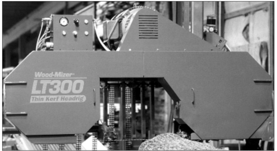
Wood-Mizer LT300 thin kerf head rig can saw both pallet and grade material.
