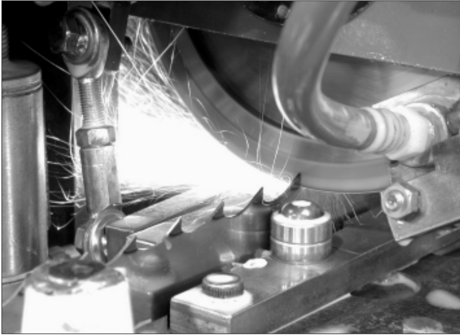
Sharpening a new blade at Wood-Mizer's plant in Indiana.
