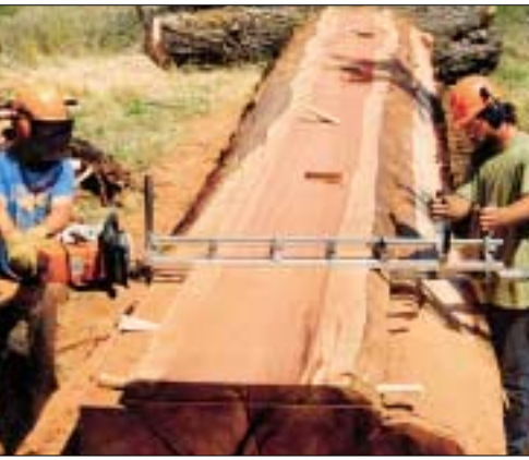
A two-man chain saw mill allows you to mill large logs and can be easier on your back.
