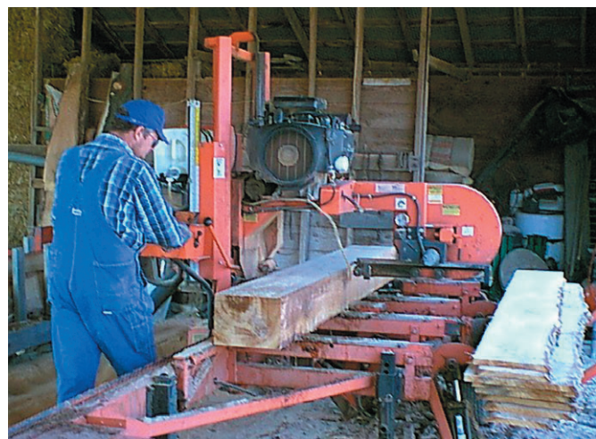
A Wood-Mizer bandsaw mill, located in an open-sided shed, makes Mark Shupe's setup complete, allowing him to cut logs into lumber before kiln drying.
